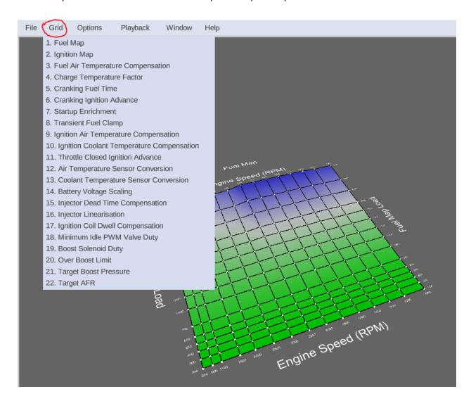
The displayed 2D or 3D grid can be panned by holding the TAB or Middle Mouse button whilst moving the mouse. In a 3D grid holding the right mouse button will rotate the map view. In order to do this the main window must be selected by left clicking anywhere in the window. A grey highlight is present around the window when it is selected.
