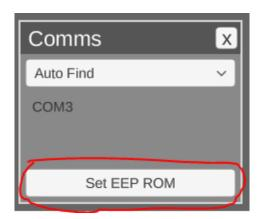
Once EEPROM saving is complete the activity indicator in the top right will flash (usually immediately unless lots of changes have been made). In addition a popup should state the save operation has completed. In some cases if a lot of data is changed 3D tuners connection may timeout. This is because saving the memory can take a long time. In this case simply wait for 3D Tuner to reconnect and the changes should be saved. To confirm you can click Set EEPROM again after it is reconnected.
