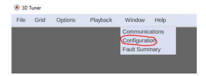
This will bring up the Configuration window which can be used to view and edit important parameters of the AugTronic ECU configuration. The parameters are split into groups and each group can be viewed by left clicking on the buttons at the top of the window. As per other windows the Configuration window can be moved and resized.
