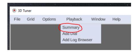
This will bring up the summary window that can be moved around the screen by left clicking and holding to the dark grey area at the top whilst moving the mouse to locate the window. It can also be resized by left clicking and holding on the icon in the bottom right whilst moving the mouse.
