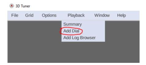
This will create a new floating Dial window that can be moved around the screen by left clicking and holding to the dark grey area at the top whilst moving the mouse to locate the window. This way a user customisable layout of key parameters can be created. Multiple dial windows can be added in this way. When the Graph checkbox is selected a graph of previous values is displayed.
