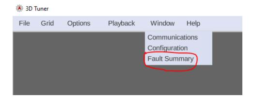
This will bring up a new window that shows the status of a number of different fault flags sent from the AugTronic ECU to 3D Tuner. When the error flag is displayed green there is no error and when it is orange an error is present. Each error has a brief description of the error, for further information on an error please contact Augment Automotive. Error flags are not stored and any error is cleared on a reset of the AugTronic ECU if the fault condition is no longer present.
